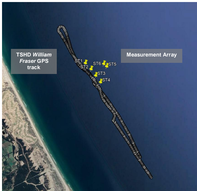
Figure 10: Google Earth image showing the GPS track of the TSHD William Fraser in relation to the measurement (hydrophone) array (ST1 through 6) on 28 November 2019 in fine weather conditions.
